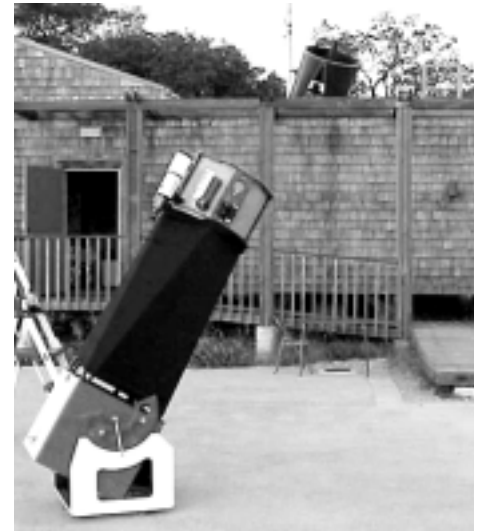
Both telescopes Jane used to observe Hickson 50 — in the foreground, the 17.5" f/4.5 Litebox dobsonian, and the 30" f/4.8 Challenger newtonian at Fremont Peak Observatory.
