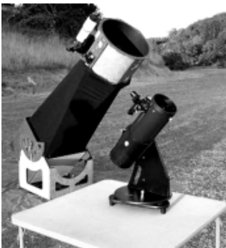
The author's 17.5-inch f/4.5 Litebox reflector "Hagrid" and 4.5-inch f/4 Orion StarBlast "Green Flash." Photo by Mike Portuesi
