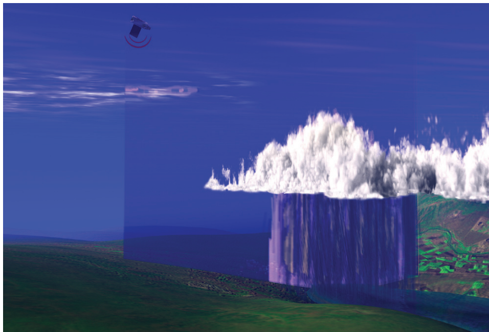
CloudSat is one of the Earth observing satellites collecting data that will help develop and refine atmospheric circulation models and other types of weather and climate models. CloudSat’s unique radar system reads the vertical structure of clouds, including liquid water and ice content, and how clouds affect the distribution of the Sun’s energy in the atmosphere. See animation of this data simulation at www.nasa.gov/mission_pages/calipso/multimedia/cloud_calip_mm.html .
