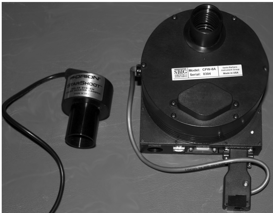
On the left is the Orion StarShoot camera, a webcam that has been packaged for use in astronomy by giving it the dimensions of an eyepiece. When purchased in 2007 the cost was $100. On the right is the SBIG ST-7X astronomical CCD imager with a color filter wheel. The 2009 price for this camera is $2495 without the filter wheel. Photo by author.
